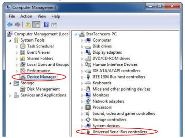
In the Device Manager, under the Universal Serial Bus Controllers category, you should see the new entries for the USB controller card.
